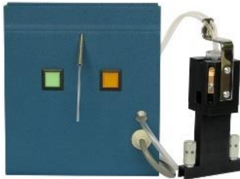
Slika 3 - 6 Pretočna kiveta s sesalno cevko v enožarkovnemu spektrometru http://www.spectrophotometer-lab.com/images/flow-through-cell.jpg (12. 12. 2010)
